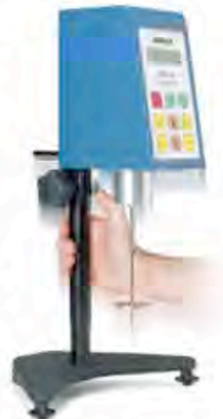
Figure 2: Brookfield Model Q Lab Stand for Rapid and Easy Movement of the Viscometer Head into and out of the Test Sample.
