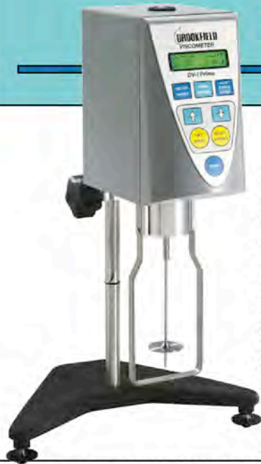
Figure 1: Brookfield DV-I Prime Viscometer with Disc Spindle used for Viscosity Check in Food QC Lab
