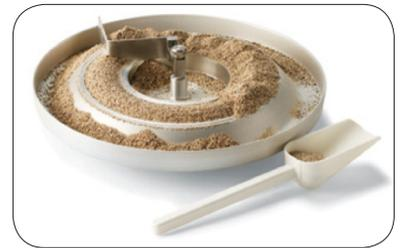
Figure 2: Shear Cell Being Loaded with Powder prior to Testing
