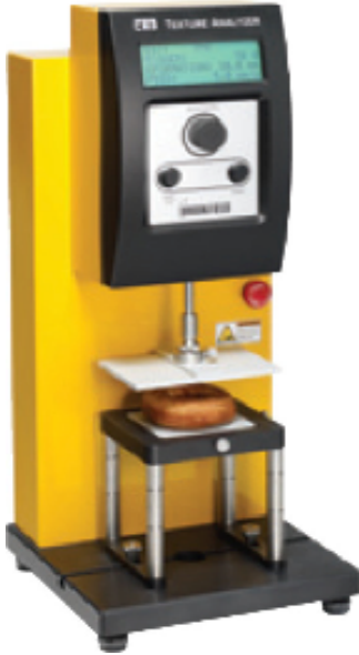
Figure 1: Brookfield's CT3 Texture Analyzer with Compression Top Plate
