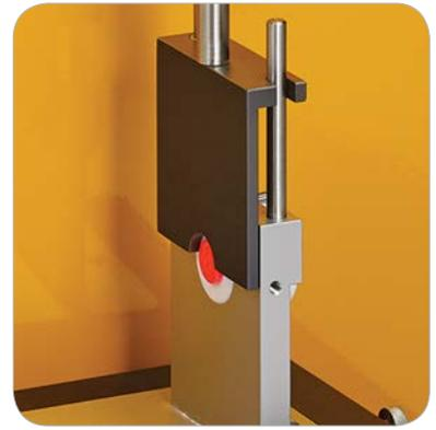
Figure 5: Blister Pack Support Test Fixture
