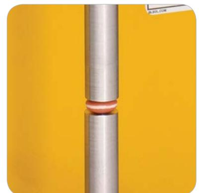
the cylinders are pulled apart and the force needed to pull the coating off of the tablet is measured.
