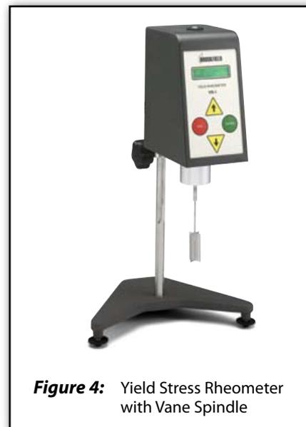
**Figure 4:** Yield Stress Rheometer with Vane Spindle
