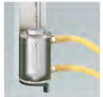
Figure 3: Cutaway of Spindle in Small Sample Adapter
