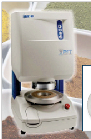
Figure 2: Brookfield's Powder Flow Tester Shear cell with powder sample
