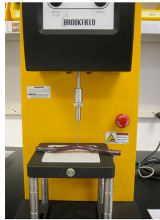
Figure 1: Texture Analyzer with probe used to compress or penetrate the sample
