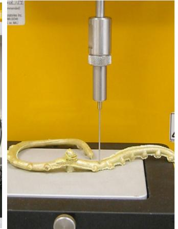
Figure 2: Shows the amount of force it will take to compress and hook fish bait
