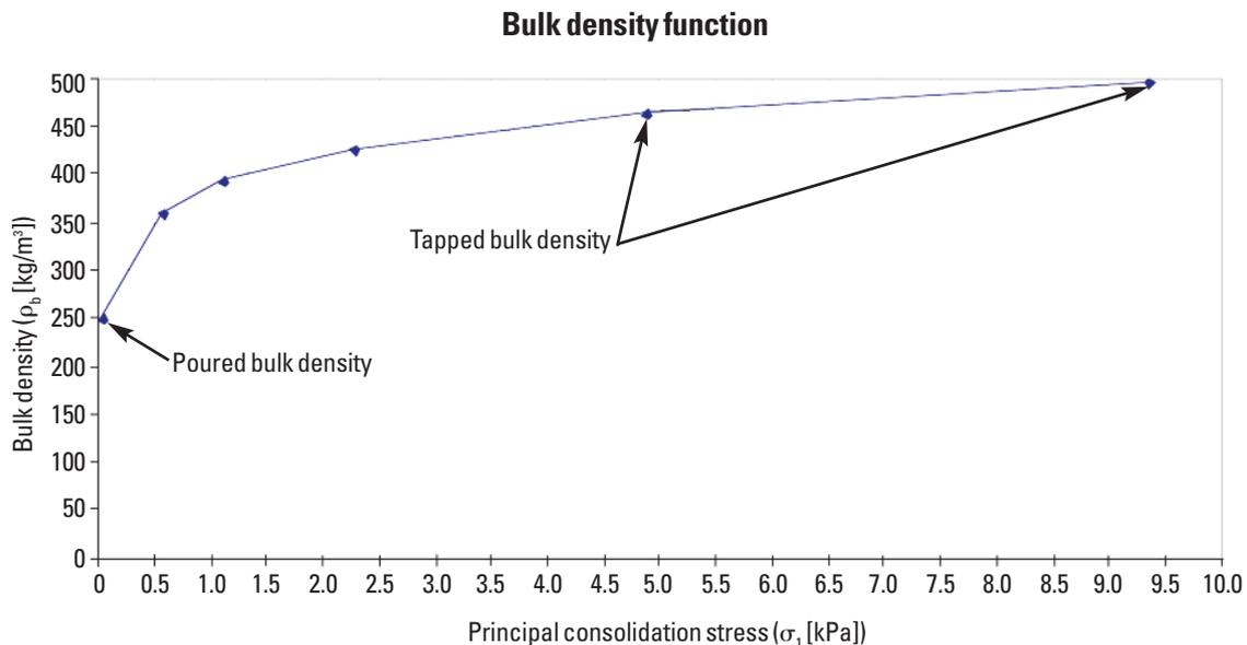
obtained at the highest consolidation load by the shear cell tester can be compared with the final density value obtained in the tap density test; ultimately, this could allow the shear cell tester to replace the lab's tap density test, saving time for the operator and better meeting the plant's needs for timely flow data.
