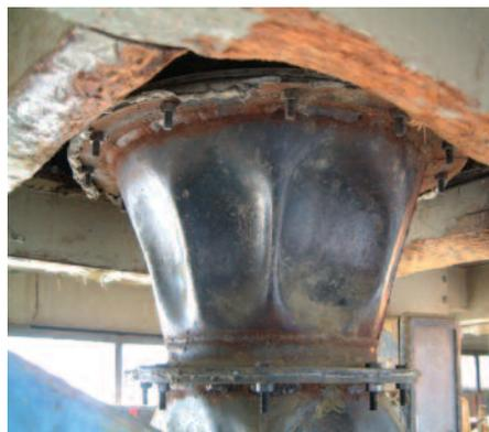
***This hopper has come down with a bad case of hammer rash — an all-too-common result when plant personnel fail to understand a powder's flow behavior.***
