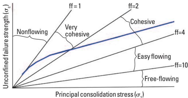
tries about what zones on the flow function characterize different flow behaviors. These zones, as shown on Figure 4, are *nonflowing* (flow function  $[ff] < 1$ ), *very cohesive* ( $1 < ff < 2$ ), *cohesive* ( $2 < ff < 4$ ), *easy flowing* ( $4 < ff < 10$ ), and *free-flowing* ( $10 < ff$ ).
