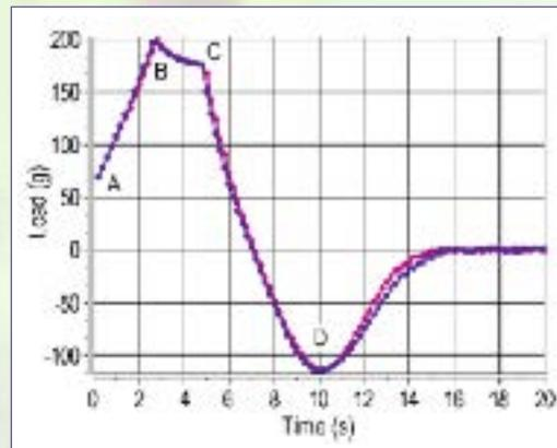
Figure 1 – A load/time graph for the adhesive force of two similar transdermal patches tested at room temperature.
