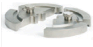
Figure 3: Custom-Design Clamshell Weight That Fits on 600mL Beaker
