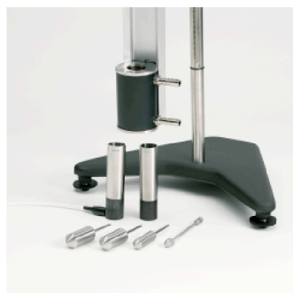
Figure 2 Spindle and Chamber Choices for Small Sample Adapter
