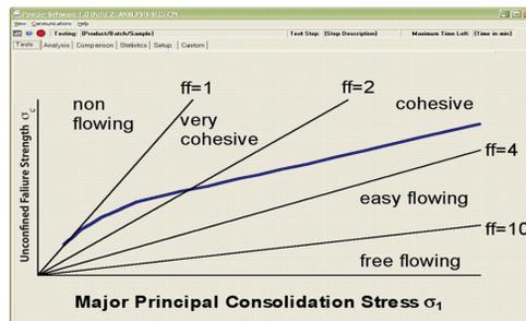
Figure 3: Graph Shows Standard Flow Function Test Data and Regions of Flow Behavior
