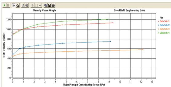
Figure 2: Density Graphs Shows Density vs. Consolidating for Different Powders
