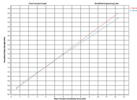
Figure 4: Graph for Quick Flow Function Test (Two Points) vs. Standard Flow Function Test (5 Points)
