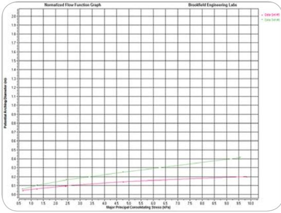
Figure 4: Comparison of Two Normalized Flow Functions
