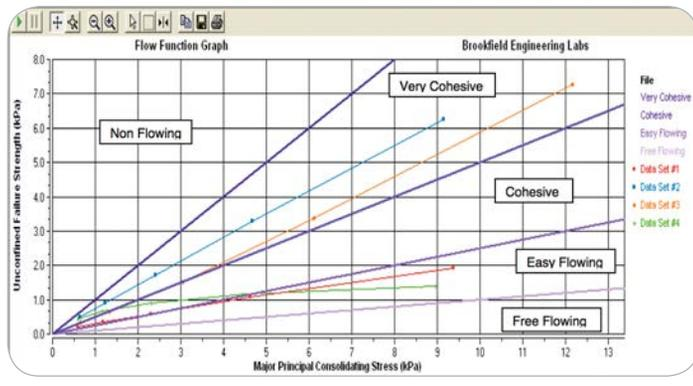
Figure 2: Standard Flow Function with Regions of Flow Behavior
