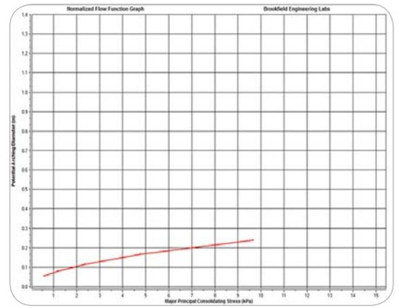
Figure 3: Graph of Normalized Flow Function Shows Arching Dimension vs. Consolidation Stress
