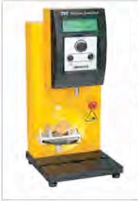
Figure 3: Brookfield CT3 Texture Analyzer with Three-Point-Bend Test Fixture for Snap Test on Crackers
