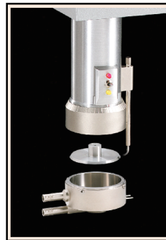
Figure 4 / Cone/Plate Spindle Geometry for Measuring Viscosity of Small Sample Volumes
