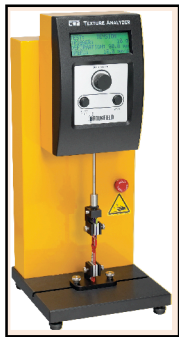
Figure 6 / Texture Analyzer with Dual Grip Assembly Measuring Force Required to Pull Apart Packaging Seal
