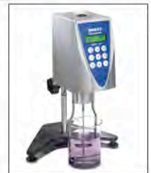
Figure 3: Standard Disc Spindle in 600 mL Beaker
