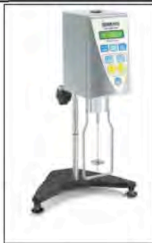
Figure 2: Standard Benchtop Rotational Viscometer for Packaging Materials
