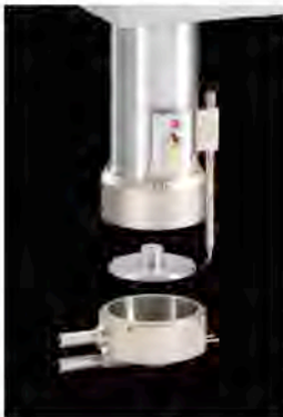
Figure 4: Cone/plate Spindle Geometry for Measuring Viscosity of Small Sample Volumes
