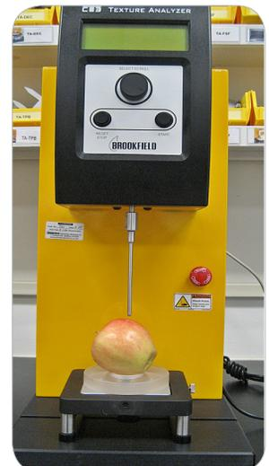
**Figure 2: Texture Analyzer with Magness Taylor Probe Positioned above Test Apple**
