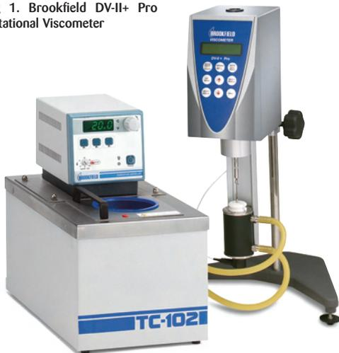
The necessity of measuring paint viscosity is well known and there are several methods using a rotational viscometer, such as ASTM D2196, for accomplishing this (see figure 1). The objective is to characterise the shear sensitivity and time dependent behaviour of paints during their application and recovery on different types of surface.
