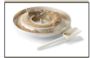
Figure 3: Shear Cell Being Loaded with Powder prior to Testing
