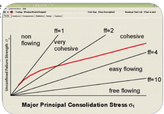
**Figure 5: Flow Function Shows Failure Strength vs. Consolidating Stress**
