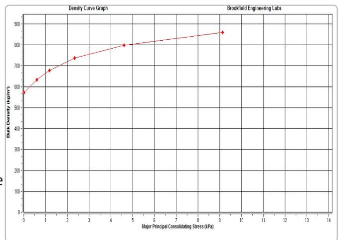
**Figure 4: Graph of Powder Density vs Consolidating Stress**
