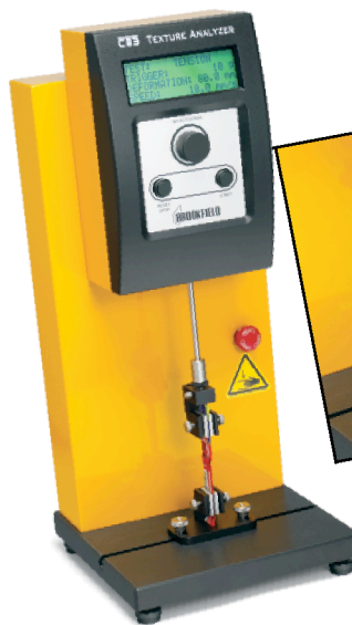
Figure 1 Brookfield CT3 Texture Analyzer with Tensile Grips
