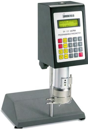
**Figure 1 /** Wells/Brookfield DV-III Ultra Cone/Plate Rheometer
