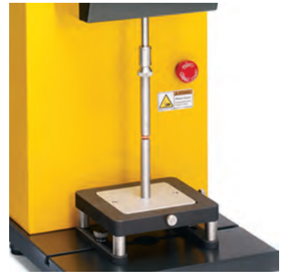
Figure 5: Brookfield RS Cone Plate Rheometer Measures Flow Behavior of Ointments
