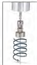
Figure 4: T-bar Spindle Cuts Corkscrew Path into Paste-Like Materials
