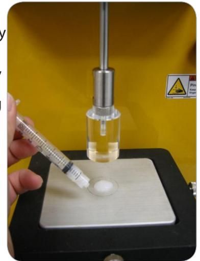
Figure 2: Sample Is Placed Onto Base Table
