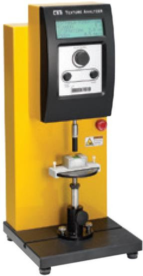
Figure 1: Brookfield CT3 Texture Analyzer Measures “Stickiness”
