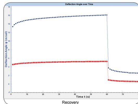
Figure 3: Creep and Recovery Graph for Two Different Materials
