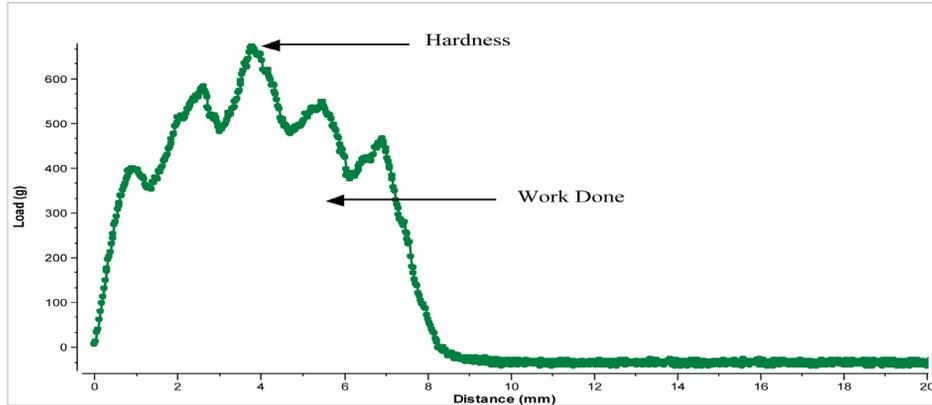
**Figure 3: The Load versus distance graph for the seal strength of a pepper sachet .** This is an alternative option of displaying the graph. Here the peak force and work done to weaken and tear at the seal is measured. The work done is measured as the area under the graph.
