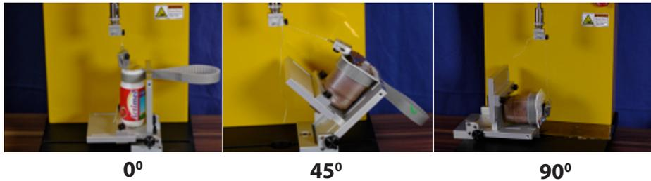
In preparation for the test, the free end of the flexible material (backing, film, etc) is inserted into the grip (or partially peeled prior to inserting into the grip) and the product (e.g., the non-flexible material) is locked into position on the
