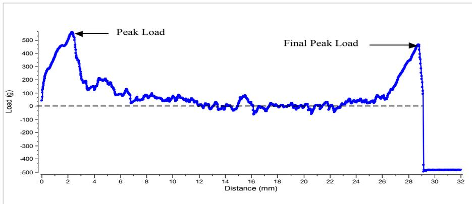
**Figure 6: The load versus distance for the peel strength of seal from a yogurt drink bottle.** This is an alternative option for displaying the results. The graph shows the distance travelled throughout the peeling process. The average peak load can however only be calculated from the load/time graph as the calculation involves a time period.
