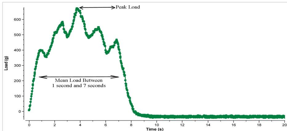
**Figure 2: The Load Verses time graph for the seal strength of a black pepper sachet.** As the tensile force increases the seal begins to be weakened at various points seen by the fluctuations on the load values on the graph. The maximum force value on the graph is a measure of the force required to initiate tearing at the seal. When the
