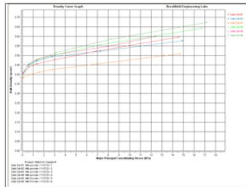
This bulk density graph illustrates the density of the samples over different consolidating stresses. All 6 milk powders show a moderate to high degree of compressibility. Loose fill density values start between 0.38 and 0.41 g/cm³. Milk powder 3 shows the least change, approximately 45%, while Milk Powder 6 shows the greatest change, approximately 70%. Powders with the greatest amount of change in density are more likely to exhibit flow behavior problems.
