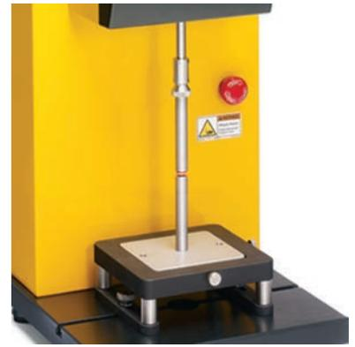
Figure 5: Brookfield RS Cone Plate Rheometer Measures Flow Behavior of Ointments
