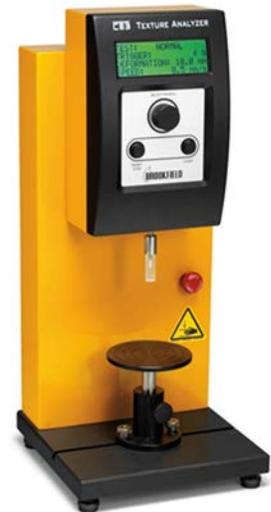
Figure 3: Test Fixture Measures Capsule Wall Strength
