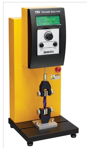
**Figure 2: Quick Test for Measuring Bonding Strength of Glue**
