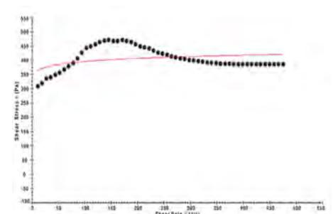
Viscosity “flow curves” are generated by testing the ointment over a range of shear rates, using the shear rate ramp mentioned above. Typical flow behavior for ointments exhibits very high viscosity values at low shear rates and decreasing viscosity values as the shear rate increases. “Pseudoplastic” is the term used to describe this phenomenon. Figure 4 shows a viscosity flow curve for a commercially available ointment.
