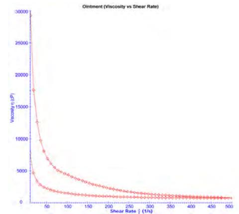
**Figure 5: Graph of Data Used to Calculate Thixotropy of the Ointment**
